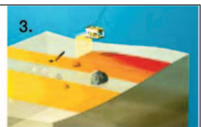
3. In 2008 a 25 metre corridor for each pipeline was inspected with high resolution equipment. Potentially dangerous objects were evaluated by independent experts.
